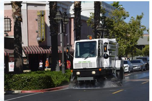
With travel speed of 25-MPH and a battery operational range of 9-11 hours, towns, villages and large cities will be able to clean the streets while protecting our environment and building a cleaner future with ZERO EMISSIONS. At the end of the shift just plug in the sweeper, recharge the batteries and sweep again.
