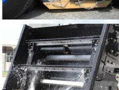
HEAVY SWEEP PACKAGE Elevator Type: Standard 11 Flight squeegee with replaceable corded rubber tips; Continuous molded rubber belts combine with standard Heavy Sweep Package make Electric Global M3 the logical choice for sweeping heavy debris such as road millings, sand and gravel up to **3-tons per-minute**. That Is one ton of sand every 20 seconds! Standard leaf gate system assists in picking up large debris, bottles, large branches and leaves.
