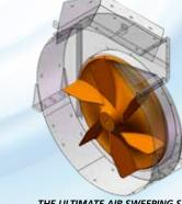
THE ULTIMATE AIR SWEEPING SYSTEM Large 32" Diamater steel Impeller includes wearresistant coating. The Internal Impeller Housing components include Rubber Lining. Driven Hydraulically. Impeller will reach speed of 3,000 RPM independent of Engine RPM or Sweeping Speed.
