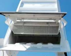
LARGEST HOPPER IN IT'S CLASS Global R4AIR includes a 5.8 cu/yd 100% Stainless Steel hopper construction, Cyclone Type Dust Separators and Swing-Down Hopper Screens are easy to clean.
