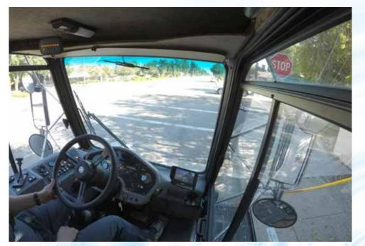
THE BEST TURNING RADIUS & EXCEPTIONAL VISIBILITY With the center mounted cab/forward layout the operator has unsurpassed visibility of the road surface as well as pedestrians and surrounding traffic. The 130-inch wheelbase allows for the sweeper to reach a turning radius of 18 1/2', wall-to-wall. With the pickup Head in the center you don't have to worry about what is happening behind you. The Global R4AIR's exceptional visibility increases operator and pedestrian safety.
