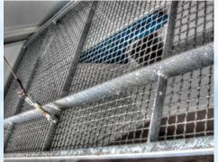
can be easily lowered for cleaning without raising the hopper. The Screening system is designed so that Hopper Screens do not plug up when sweeping light debris such as leaves.
