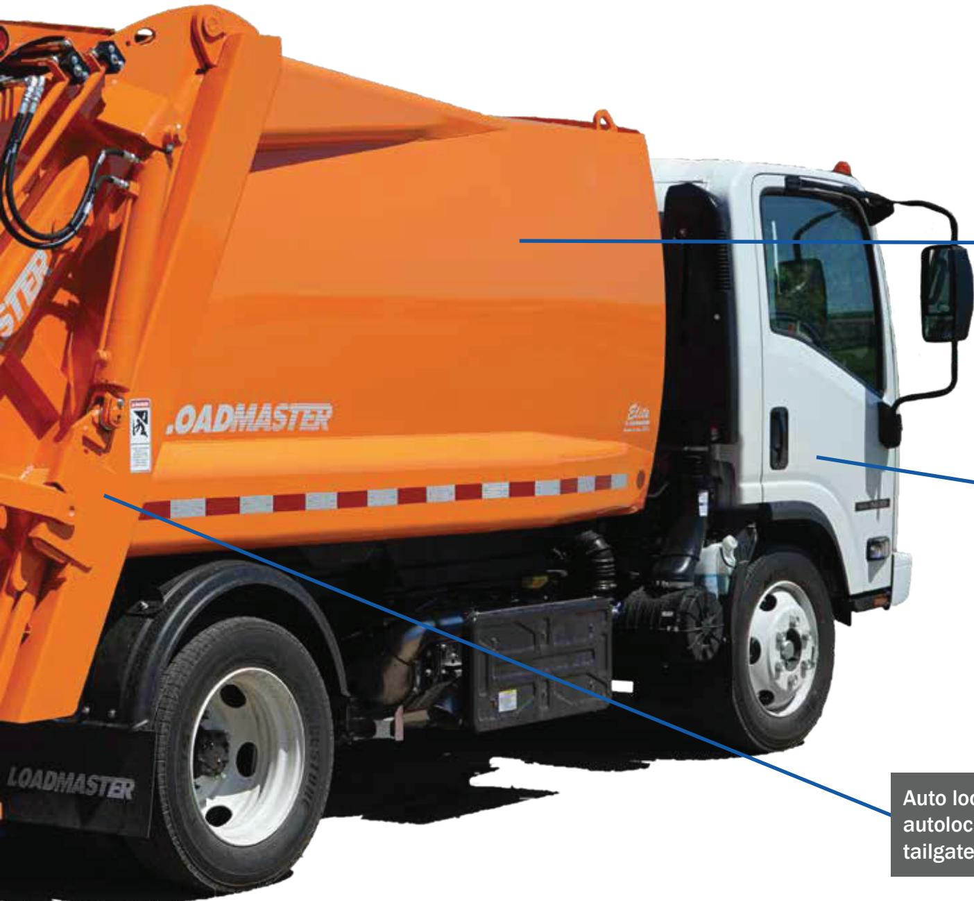
Strong, smooth, curved 10 gauge high tensile body sides. Designed to look good on any chassis. The smooth sides provide a good surface for decals, signs and other advertising. 10 ga high tensile body sides, 10 ga high tensile body roof, 3/16" body floor.
